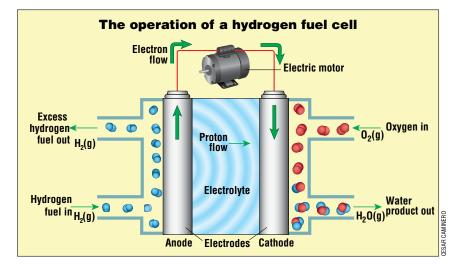
Hydrogen ions are formed when electrons are removed from  $H_2$ . The electrons move through the circuit to the cathode–causing the motor to work in the process. The hydrogen ions combine with  $O_2$  gas to form water.
